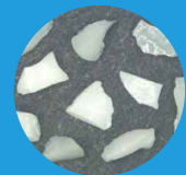
Macrostructure of 36-grit Weak Splintery-shaped CERPASS XTL™-0565 grains.
