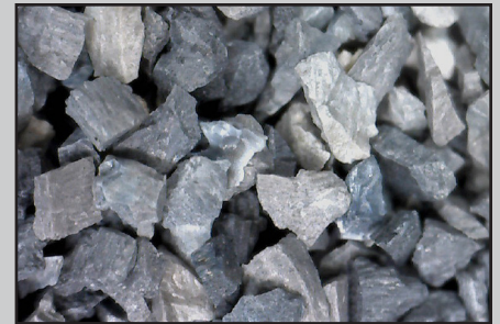
Macrostructure of AZ-40 grains
