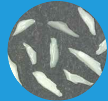
Macrostructure of individual Extra Sharp exploded CERPASS DGE™ - 0123 grains.
