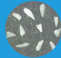
Macrostructure of individual Weak Splintery-shaped CERPASS XTL™-0570 grains
