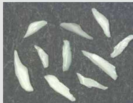
Macrostructure of individual Extra Sharp exploded CERPASS DGE®-0123 grains.
