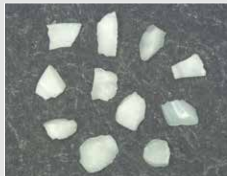
Macrostructure of 36-grit CERPASS HTB® grains.
