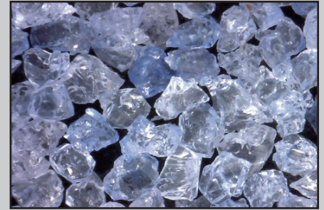
Macrostructure of MA88K grains
